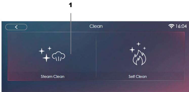
The **steam cleaning function** assists in removing food residue and grease from the walls of the oven. This function is the best for light stains. In cases where fundamental cleaning is needed, the high temperature self-cleaning function is required.
