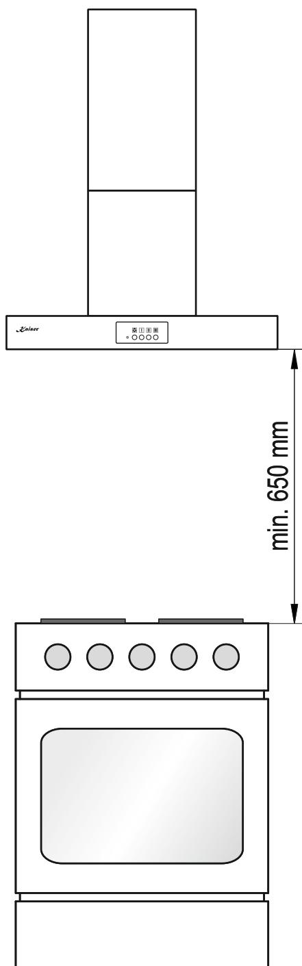
The cooker hood was designed for removal of kitchen fumes to the outside. It should be connected to an appropriate ventilation duct (do not connect the hood to any chimney, smoke or flue-gas ducts which are in use).
