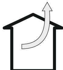
In the extractor mode air is discharged to the outside by a special conduit. In that setting any charcoal filters shall be removed.
