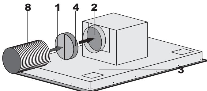
If the V-Flap **1** is not installed on the air outlet **2**, it should be mounted
