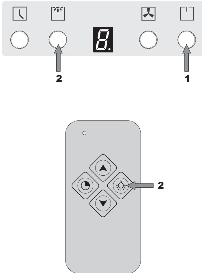
The remote control has to establish a new connection to the cooker hood when it is used for the first time. One remote control could control several cooker hoods at the same time.
