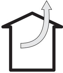
In extractor mode the air is discharged to the outside by a special conduit. Remove any charcoal filters in case if they have been installed by factory (see **Replacement of the filter**). This increases the performance of the cooker hood.
