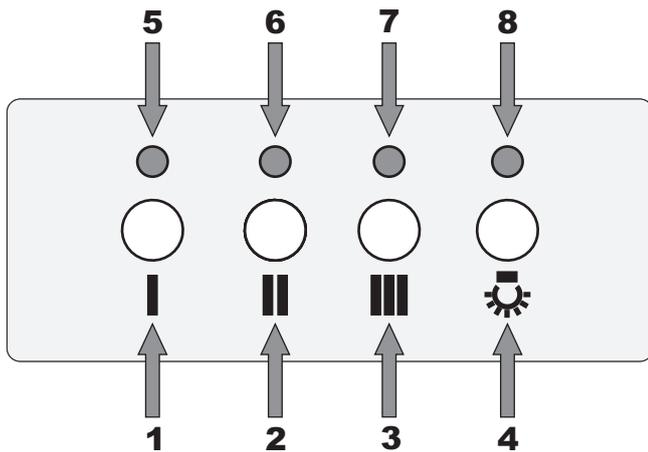
According European Norms 65/2014 and 66/2014 the hood with motor power more that 260W may work on high speed **III** only 7 minutes, after 7 minutes the speed is changed to medium speed **II** automatically.
