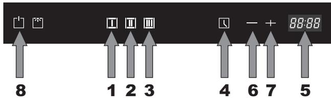
During the timer cycle the cooker hood functions with chosen speed.
